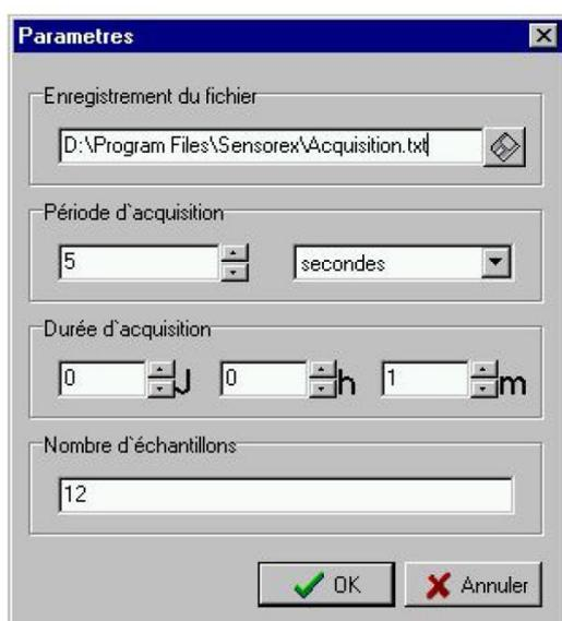
figure 6 : Configuration de l'acquisition.
