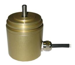
Meggitt (Sensorex) (IS) SX36RV provides a sinusoidal signal, with a linear voltage over the measurement range. The primary is excited by an AC voltage, and is picked up by the secondary winding on the transformer principle; the position of the rotating core determines the transformer ratio of each secondary winding.
